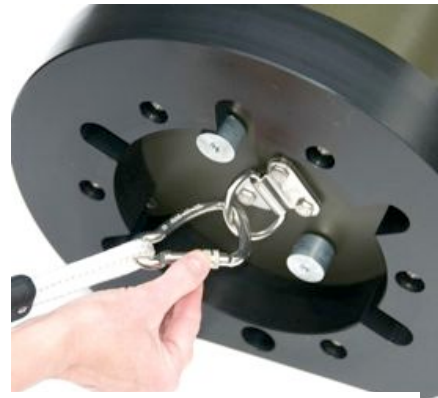
Figure 5. Attach stability weight to the bottom eye with locking carabiner.
