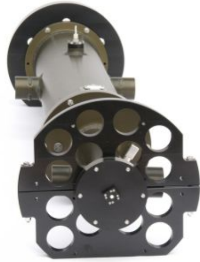
Figure 2. WaLRUS resting safely on its side, with the top-mounted Ed collector and protective plastic ring in the foreground
