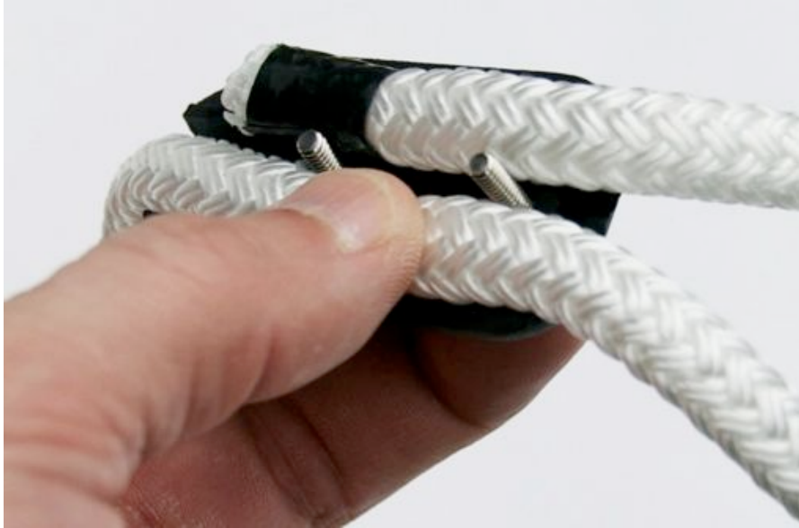
Figure 9. Assembling a rope clamp. First place the rope in the half of the clamp with unthreaded screw holes. Hold the screws in place while place the other half (not shown) on top. Then tighten the screws.
