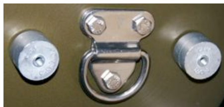
Figure 12. Two round zinc anodes protect the other metal parts from corrosion.
