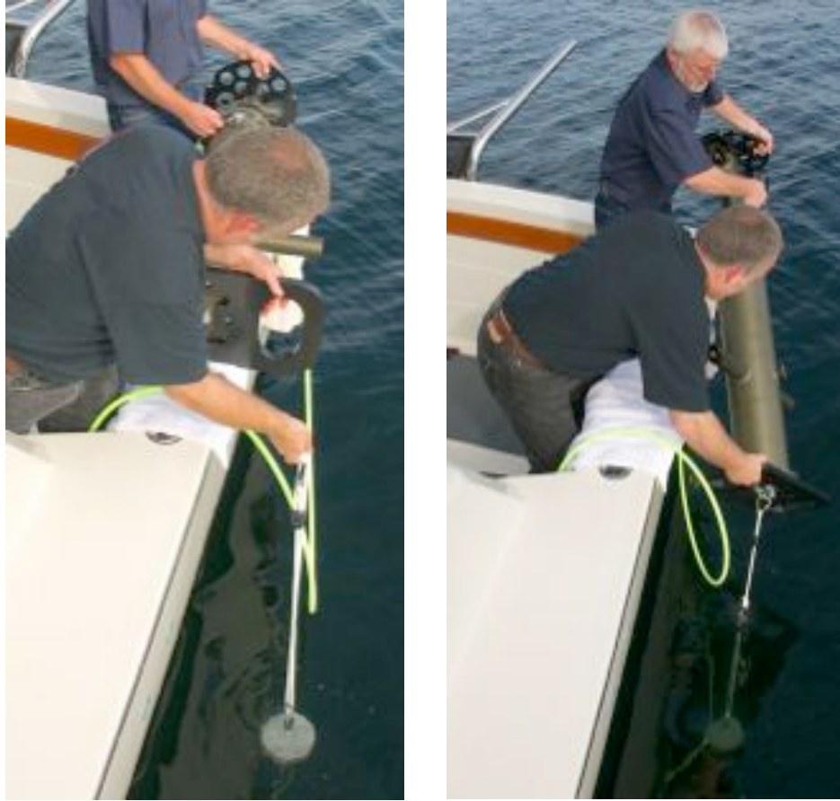
Figure 6. To deploy, lower the stability weight into the water while holding the WaLRUS on deck. Then lower the WaLRUS.
