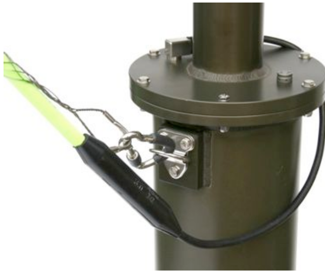
Figure 4. Proper attachment of tether, with loop for strain relief.
