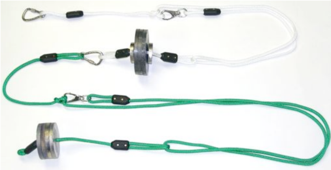
Figure 7. Weights and ropes for profiling. Upper weight with white ropes is stability weight. Lower with green rope is profiling weight. Adjust rope lengths by adjusting the loops, as shown in Figure 8 .
