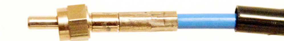
SMA termination with boot removed
