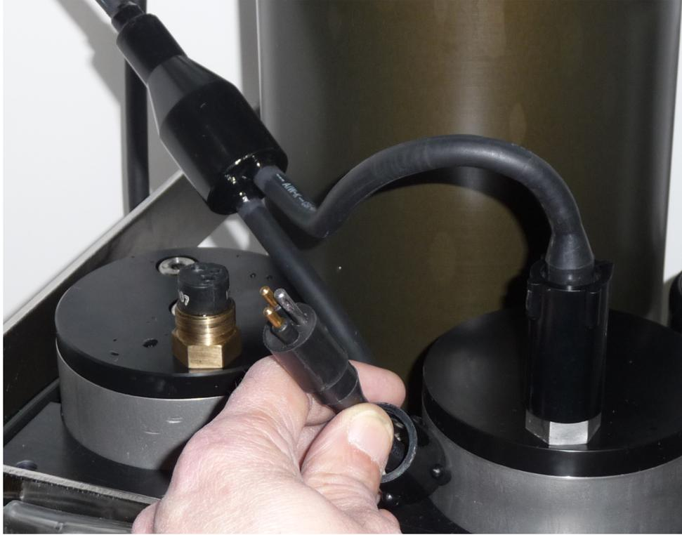
**Figure 4. Beware: when one leg of the Y is plugged into a pack, the second plug is live.**
